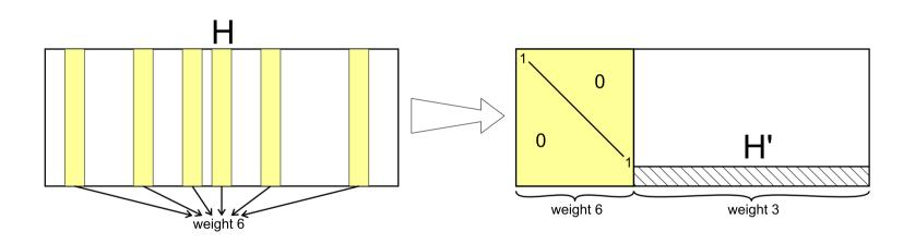
$\Rightarrow$  We decode 3 errors in a shortened code. The parity check matrix H' of this code is obtained by applying a Gaussian elimination to H (about  $2^{24}$  column operations).
